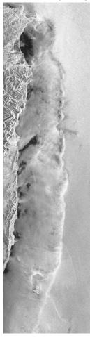
The ERS-2 SAR image depicted in Fig.1 shows a frontal line along the east coast of Taiwan at a distance approximately 50 km offshore. In the lower (southern) section, the image intensity, and thus the small-scale sea surface roughness, is strongly enhanced in the frontal area due to flow convergence caused by opposing winds. The semi-circular features with dark patches in the middle visible in the upper (northern) section of the image are sea manifestations surface of convective rain cells.
