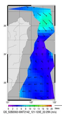
Figure 6. Wind field map derived from Quikscat data acquired on 7 January 2002 at 05:42 LT.
